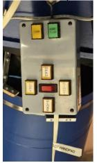
The dome can also be rotated by using the button and switch located on the dome motor control box.
