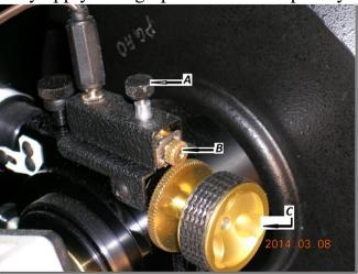
3. Adjust the Celestron telescope focus using the knob located on the telescope visual back until you attain a rough focus.
