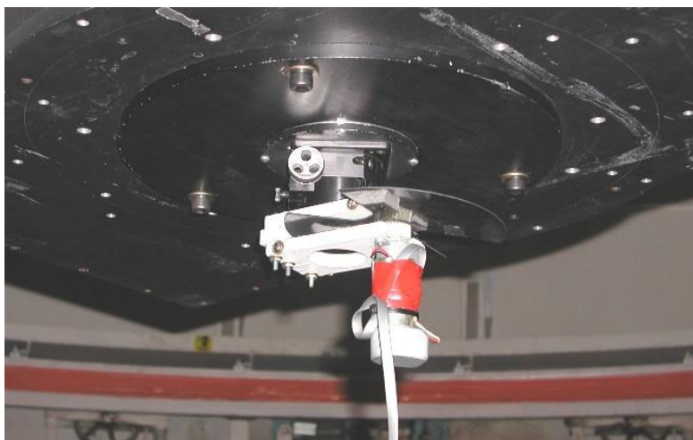
Picture above is the “chopper” mounted to the 61” Kuiper Telescope
