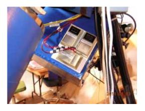
Another safeguard employed is the addition of sensing relays into the power supplying the servo controller and the viewing deck pier boxes. If any of these 12 Volt DC supplies is left energized, the building alarm system can't be activated.
