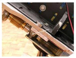
The final problem encountered was that of balance. Once all the peripheral equipment was mounted to the telescope, the RA and Declination gears were disengaged to allow free telescope motion in all directions. Counterweights installed and positioned in the proper locations allowed the telescope to be precisely balanced in X, Y, and Z axis.
