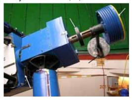
To prevent damage to the telescope, limit switch circuits were designed and installed. The RA limit switches mounted on the axis tube prevent the telescope from continuously rotating, a situation that would damage the cables running up the centre of the axis tube to the wiring panel. A feature built into the RA movement is a limit switch that prevents the telescope, if left unattended, from impacting the stairwell wall.
