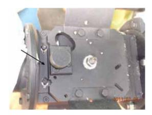
Moving along the light path from primary mirror to secondary mirror to the eyepiece, the next order of business was to replace the diagonal mirror. This is a flat piece of glass mounted to a mechanism used to select, via the central knob viewable in the accompanying image, one of the four viewing ports available on the rear of the mirror box.
