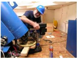
To remedy the issue of inaccurate RA gear plate to worm gear alignment resulting in binding and excessive gear tooth wear, the RA motor assembly was retrofitted with a calibration plate. Using this plate and a set of calipers, the angle of contact can be precisely set to ensure correct meshing of the RA plate teeth to the worm gear. The distance requirements are displayed on the plate for easy reference.
