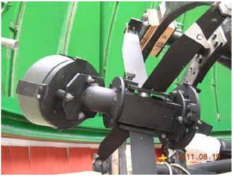
This manually operated assembly holding the secondary mirrors allows a user to choose how to use the telescope. The f12 Cassegrain mode lets a person use the telescope visually, and to date has been very popular with both members of the Centre and the general public. Choosing the f4 Newtonian option permits an operator to use the new SBIG ST-10XME CCD camera and CFW9 colour wheel to photometri-
