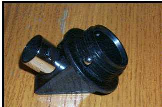
Modified 0.93" diagonal to hold 1 1/4" eye pieces
