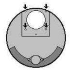
4. Using the four 4-40 by 3/16 socket screws provided, attach the *CFW-9* cover to the front of the ST-7/8/9/10/2000. Make sure you use the provided screws whose length of 3/16 is required to thread into the ST-7/8/9/10/2000 front plate without breaking through the blind taps. Then re-assemble the carousel and housing.
